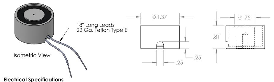
Voltage: Duty Cycle: 12 VDC Continuous
