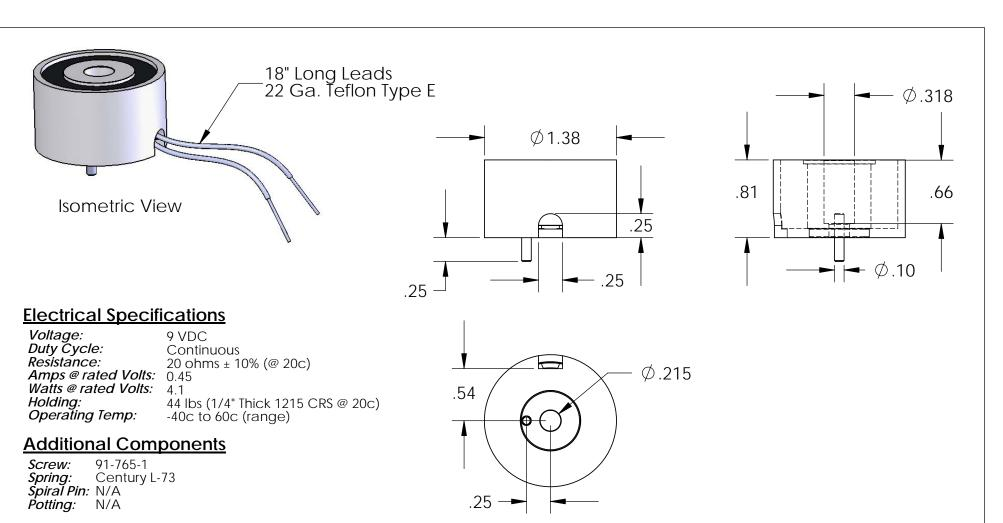
*Finish:* Housing - Zinc or Electroless Nickel Plating (0.0002-0.0003")
