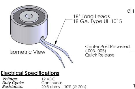
20.5 ohms ± 10% (@ 20c) Amps @ rated Volts: 0.58 Watts @ rated Volts: 7.0
