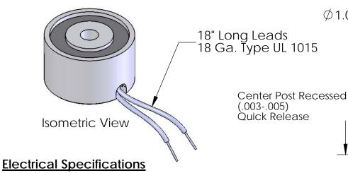
Voltage: Duty Cycle: Resistance: 24 VDC Continuous
