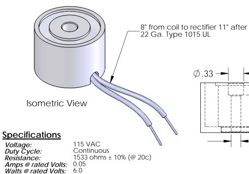
66 lbs (1/4" Thick 1215 CRS @ 20c) -40c to 60c (range) Holding:
