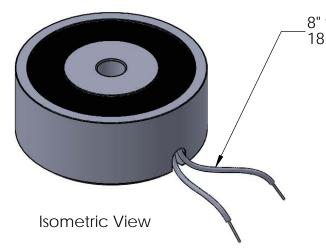
8" from coil to rectifier 11" after 18 Ga. Type 1015 UL
