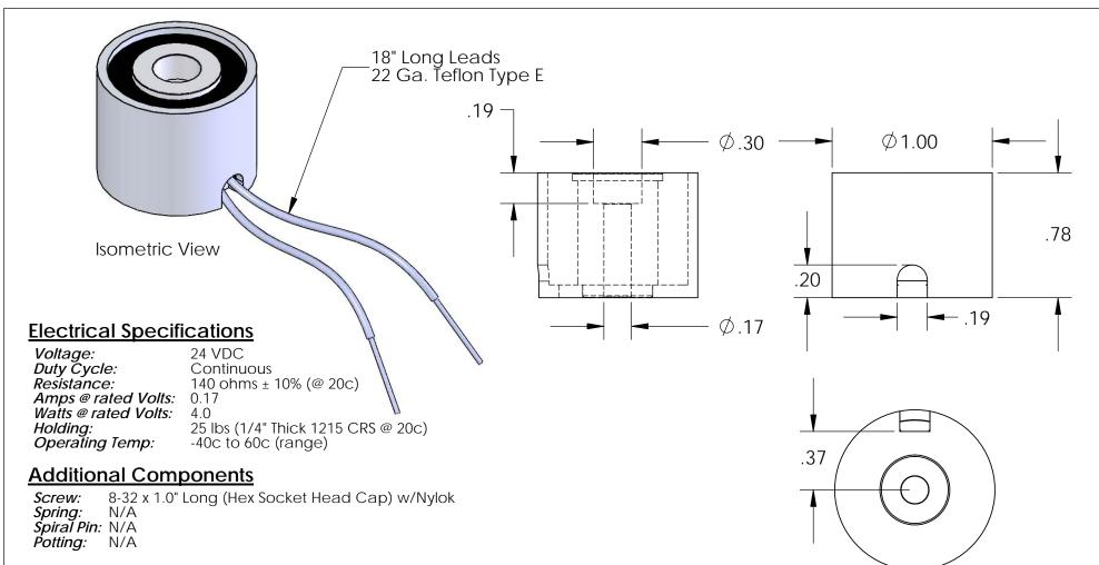
Housing - Zinc or Electroless Nickel Plating (0.0002-0.0003") Finish:
